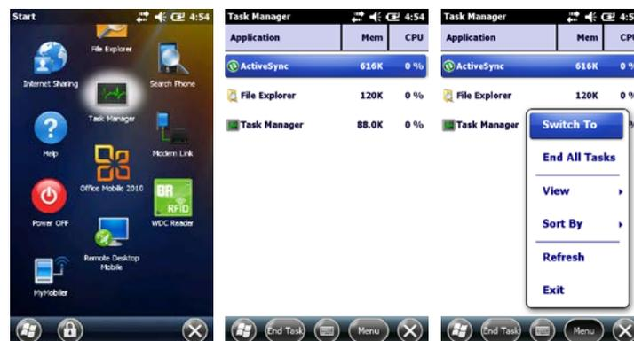
Task Manager can manage all running task on E430. Go to **Start menu > Task Manager** to open task manager program. You can tap each one task and press the **End Task** button on bottom to end it or tap **Menu** to choose **End All Tasks**.
