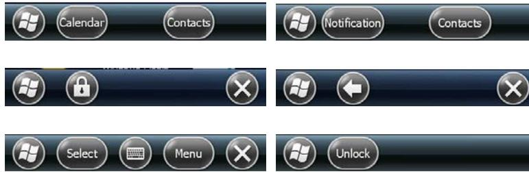
You can press to enter Start Menu. Press will back to previous step. Press to lock E430 and if you want to unlock just press to enter unlock page.
